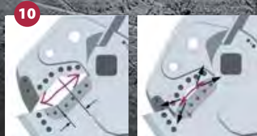
Offset APEX: Steel is compressed and molded in the mouth and thus easier to cut
