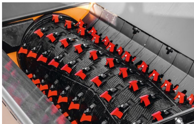
DOPLOCK FIXTURE SYSTEM Self-locking fixture system for highest stress. The bolt is just a retaining device
